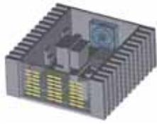
Mechanical CAD geometry defeatured and converted into Icepak objects with ANSYS DesignModeler
